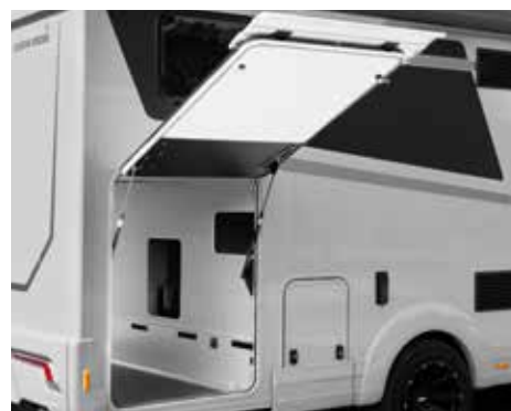
Particularly large load volume thanks to double floor height of 30 cm.
